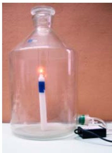
Fig.1 Photo of the short experiment: "Oxygen consumption by a candle"
