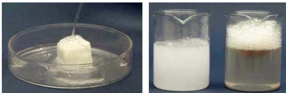
Fig.7, Fig.8 Stills from the film: Effects of hydrochloric acid on calcium carbonate and natural limestone
